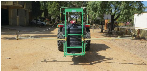
Figure 1. Rear view of the tractor-operated automatic gun sprayer
